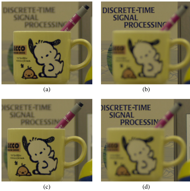
Fig. 6. Examples of captured real images: (a) A near-focused image at X=16 [mm] (b) A far-focused image at X=16 [mm] (c) A near-focused image at X=24 [mm] (d) A far-focused image at X=24 [mm]
