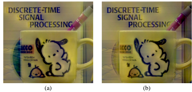
Fig. 12. Generated f'(u, v; 0.5) and f''(u, v; 0.5) that are averaged to be the final interpolated image shown in bottom-left in Fig. 10.
