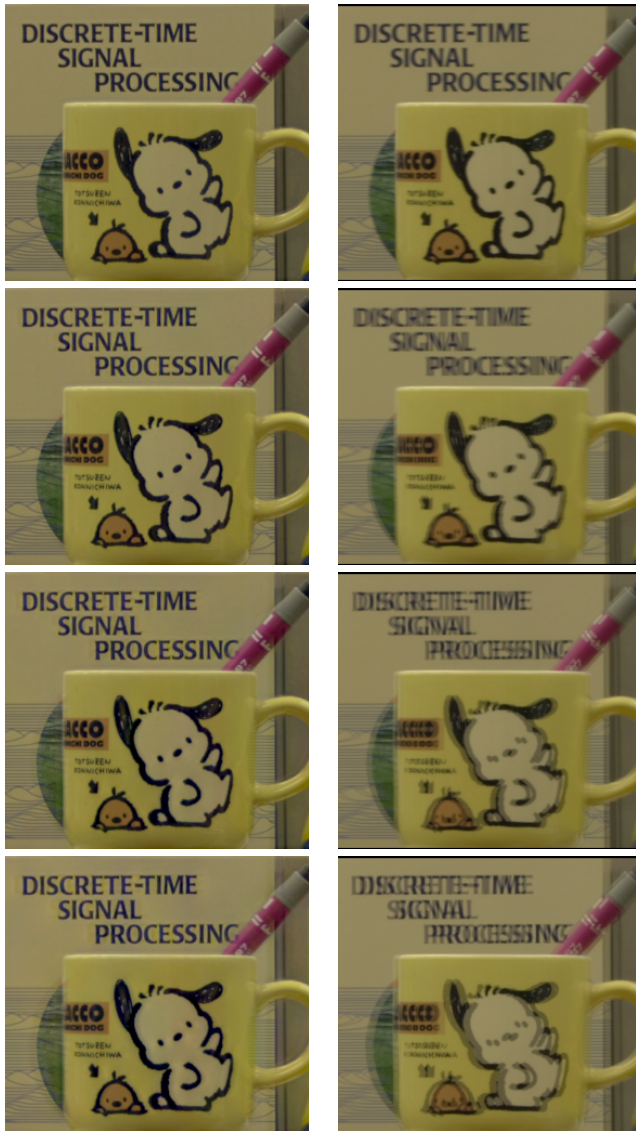
(b) Interpolated images by the proposed method (left) and LFR method (right) at the center of two cameras for various distances between cameras of 4, 8, 12, and 16 [mm] (from top to bottom).
