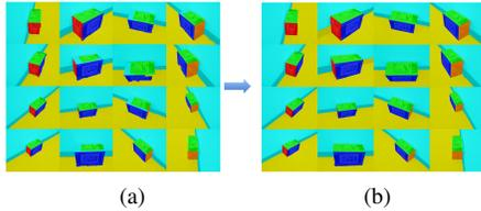
**Fig. 4:** Segmentation refinement: (a) Original segmentation of the planes with superpixel leaks (black circle); (b) Refined segmentations (Best viewed in color).
