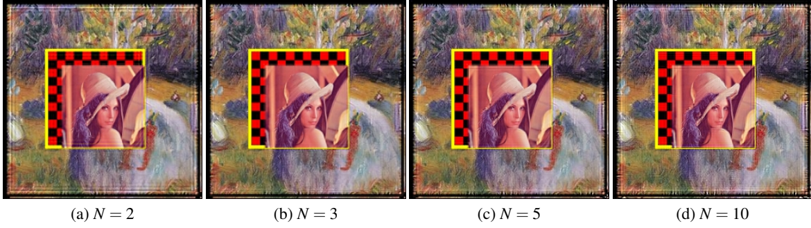
Figure 4: Effect of choosing the number of focal planes. The novel views are reconstructed by our method after 10 iterations using different numbers of focal planes.
