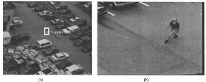
**Figure 8: VSAM [32] tracking between cameras. (a) target identified in one camera (b) a camera with a better view is maneuvered to intercept the estimated target trajectory**
