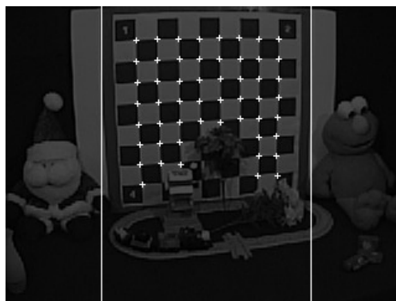
Fig. 13. Locate the feature corners of the calibration pattern.
