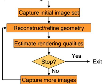
Figure 5 The flow of AIBR capturing.
