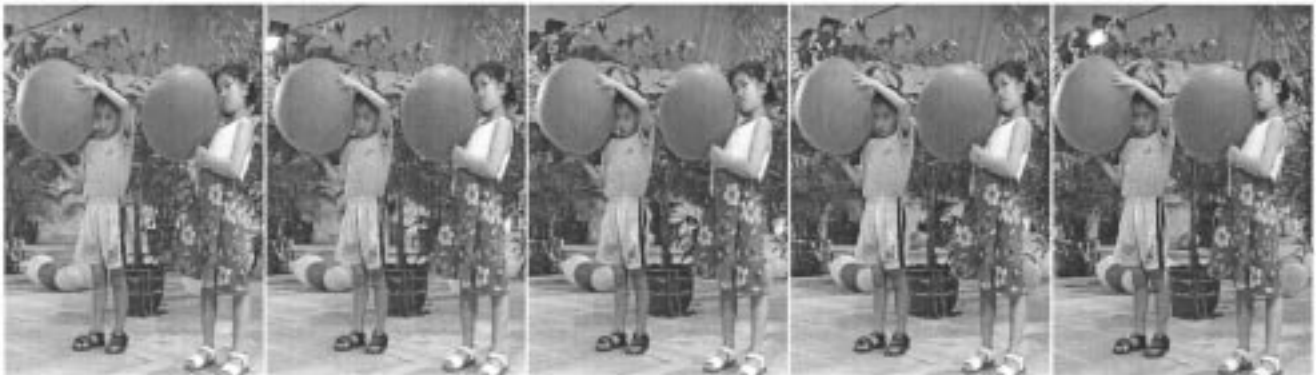
Fig. 9. Set of smartly rebinned panoramas at the same horizontal location (note the parallax shown by the lightbulb and the balloon behind the leg of the girl).
