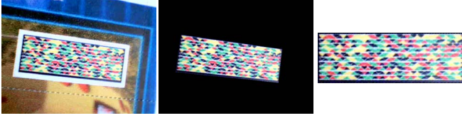
Figure 10: Left to Right: Input image, region of the input image lying within the corners localized, barcode extracted and transformed to a canonical rectangle.
