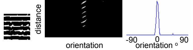
Figure 5: Left to Right: The patch extracted from thresholded image, the Hough transform of the patch, and the 1D orientation profile, obtained by summing the Hough transform along one dimension, where the peak corresponding to the orientation of the barcode is evident.
