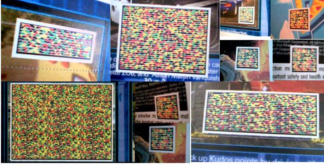
Figure 2: Example images of the Microsoft High Capacity Barcode (Viewed better in color).
