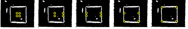
Figure 7: Left to Right: Starting with a small square around the point known to lie inside the barcode, we swipe each edge till it is mostly white. This gives us the initial rough corner estimates.
