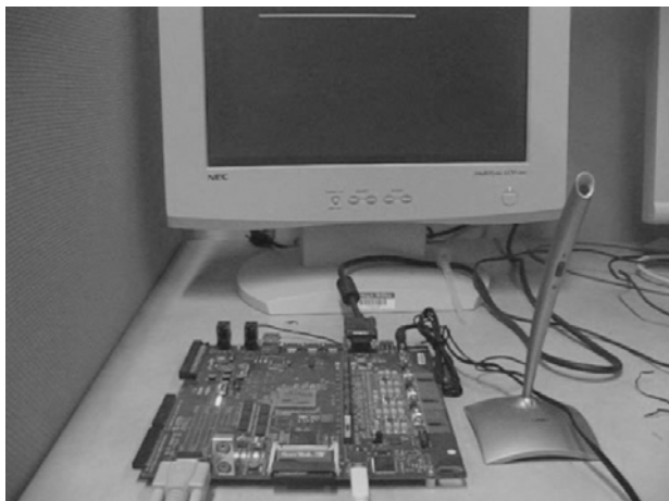
Figure 11. Fully custom hardware speech recognition system setup
