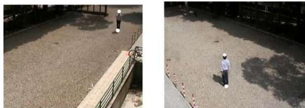
Figure 1: The proposed method uses only corresponding image points of foot and head location between cameras to compute their internal parameters and their relative position.
