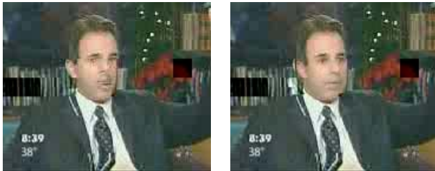
(a) (b) Figure 9. Error concealment for the Inter coding scenario with: (a) motion compensation; (b) motion compensation and UMPC
