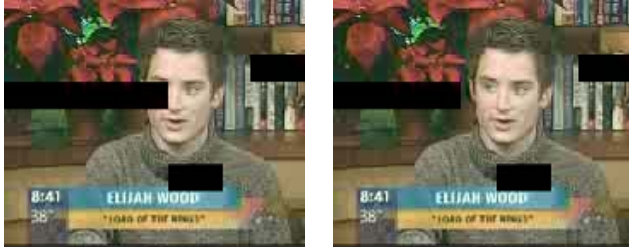
(a) (b) Figure 8 Error concealment for the Intra coding scenario with: (a) no concealment; (b) concealment with UMPC
