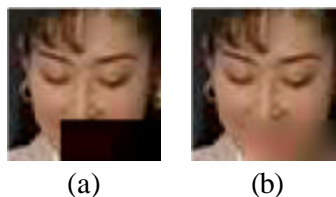
Figure 5. Error concealment example by spatial interpolation: (a) the corrupted frame without error concealment, and (b) the reconstructed frame with error concealment
