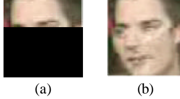
Figure 6. Error concealment example by temporal interpolation: (a) the corrupted frame without error concealment, and (b) the reconstructed frame with error concealment
