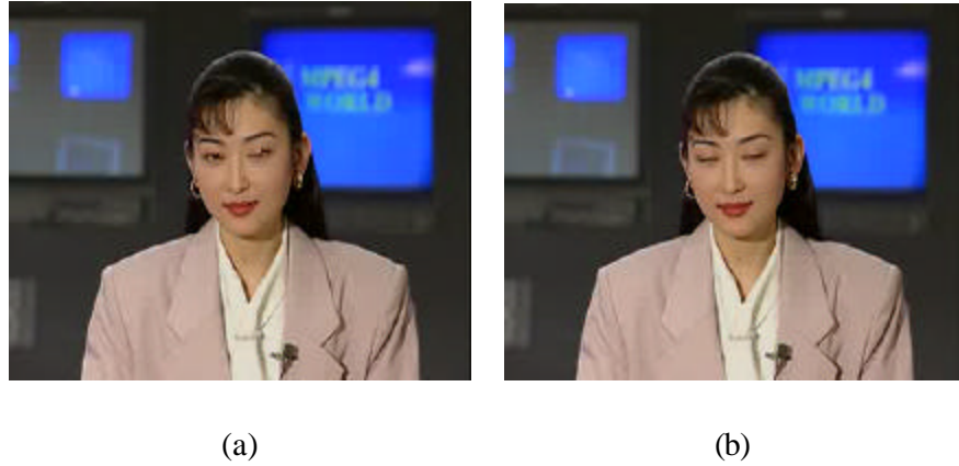
Figure 26. Example decoded frame, Frame 5, of Sequence “akiyo” with (a) UPPRS and (b) ECARS
