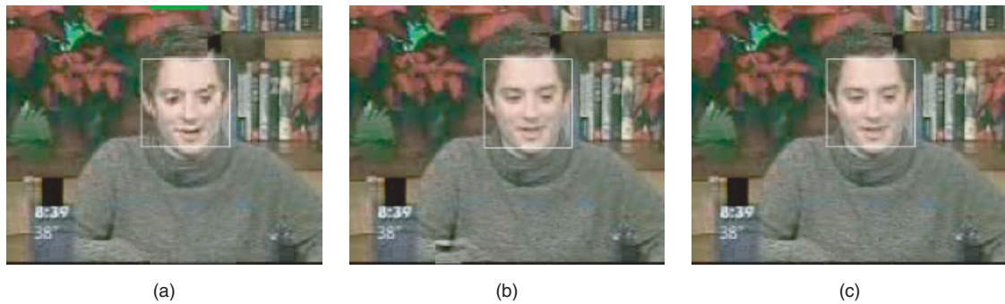
Fig. 18. Sample reconstructed frame at time 19 of Inter coded 'Interview' with MVs reconstructed by (a) spatial-nbr; (b) temporal-nbr; and (c) U-Eigenflow for MVs, followed by UPC for ROI for all three MV reconstruction methods.
