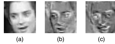
Fig. 2. PCA for face images: (a) mean; (b) first eigenvector; and (c) second eigenvector.
