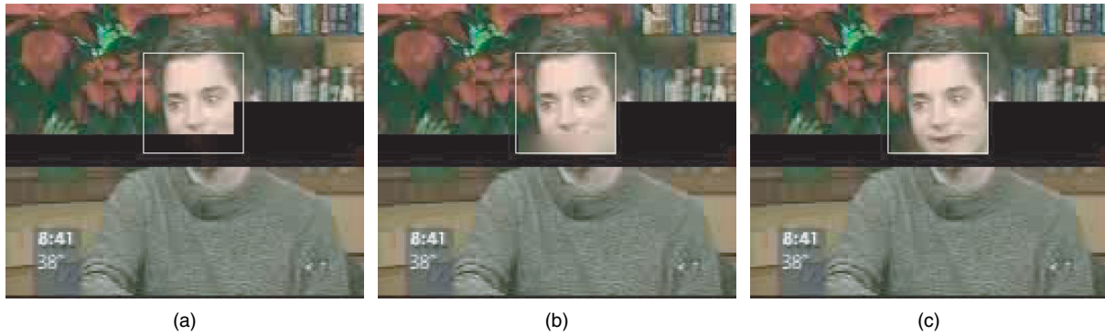
Fig. 11. Sample reconstructed frames of Intra coded ‘Interview’ with (a) no concealment; (b) concealment with spatial interpolation; or (c) concealment with UPC for ROI.
