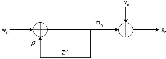
Figure 4 AR(1) model for observed samples
