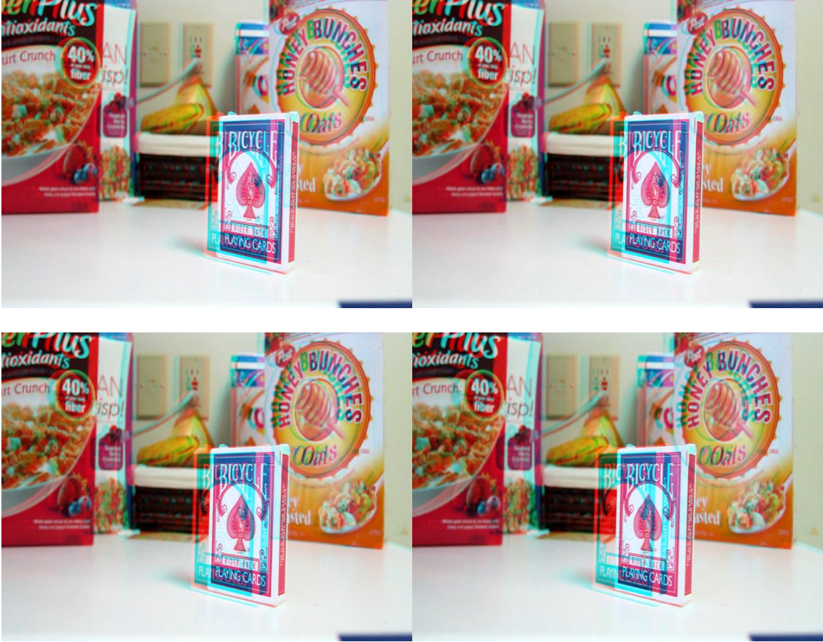
Figure 7, four consecutive frames in the output of method A using lower sampling rate data set. Notice that the distance between the two views changes a lot for different frames frame.
