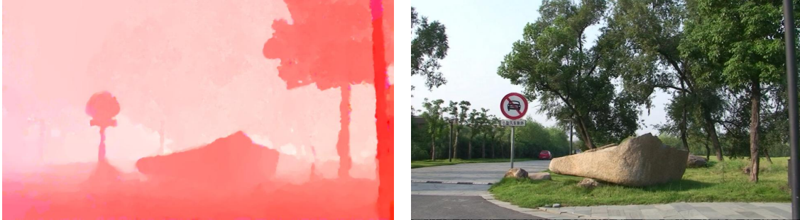
Figure 4, left: optical flow map, right: image synthesized using optical flow
