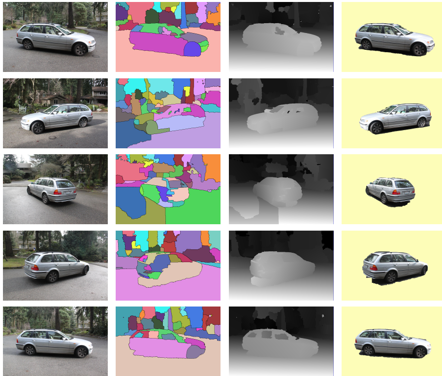
Fig. 6: CAR DATASET (Five out of 45 images): Our method handles difficulties arising from reflections in the glass windows and the specular surfaces of the car and accurately segments the car in many of the input images.
