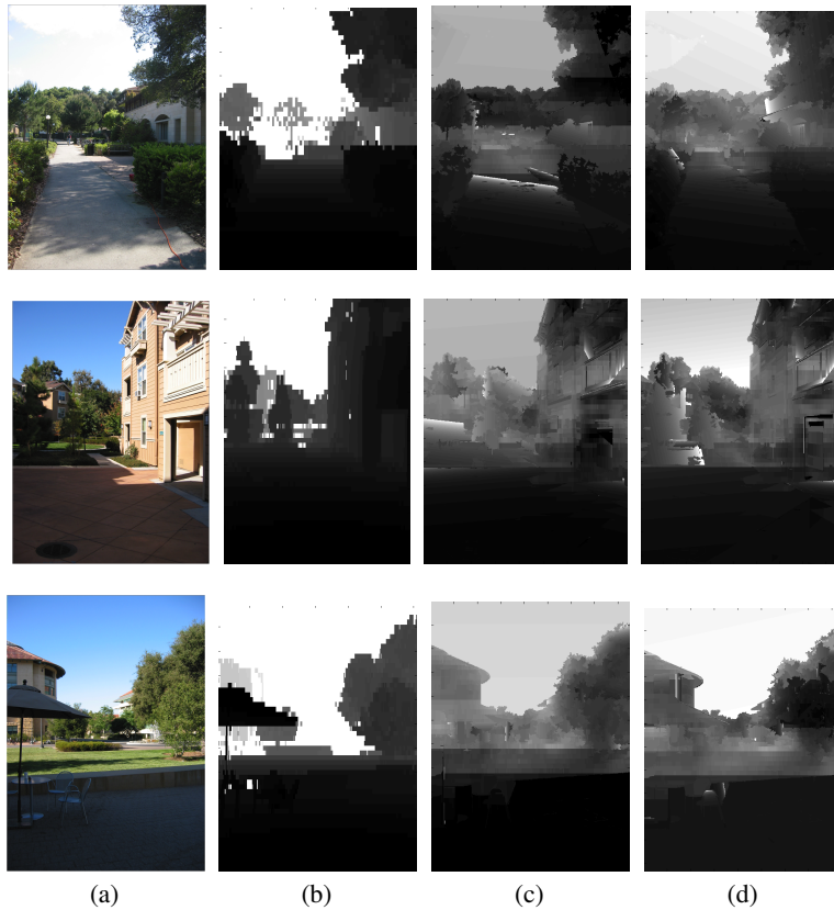
Figure 1: (a) Image from the dataset; (b) Ground truth; (c) Result obtained using CCM; (d) Result obtained using the proposed FE-CCM. (Best viewed in color)
