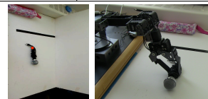
Fig. 10. Left: the grasping point detected by our algorithm. Right: Our robot grasping an object using our algorithm.
